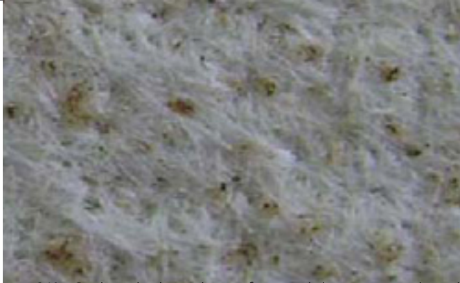
NOMEX 500 g/m2 singed 2 340°C resistant to acid dew points. High peak temperature resistance.
